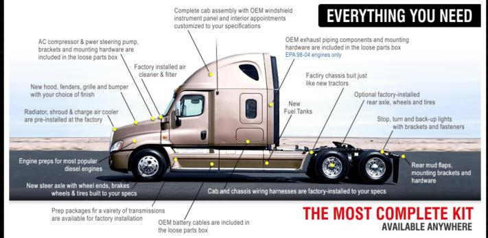
At a glance, the most seasoned trucker won't spot the difference between a Freightliner Glider Kit and a new truck. A Glider Kit comes to you as a brand-new, complete assembly that includes the frame, cab, steer axle, wheels, a long list of standard equipment and a loose parts box with up to 160 additional parts. Your Glider Kit has everything you need to hit the road in a "new" Freightliner or Western Star.
